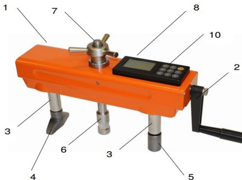
Fig. 2. General view of ONYX-1. Os. 050, ONYX-1. Os. 100 devices [1]: 1-housing; 2-drive handle; 3-hydraulic cylinders; 4, 5-supports; 6-traction; 7-steering wheel; 8-electronic unit; 9-USB connector
