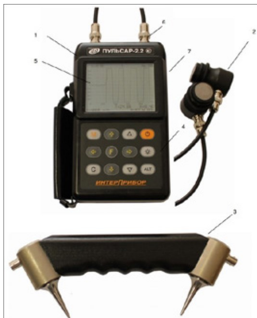
Fig. 4. General view of the PULSAR-2.2 device [1]: 1-electronic unit; 2-through-sounding sensors; 3-surface-sounding sensors; 4-keyboard; 5-graphic display; 6-connectors for the surface-sounding sensor; 7-USB connector
